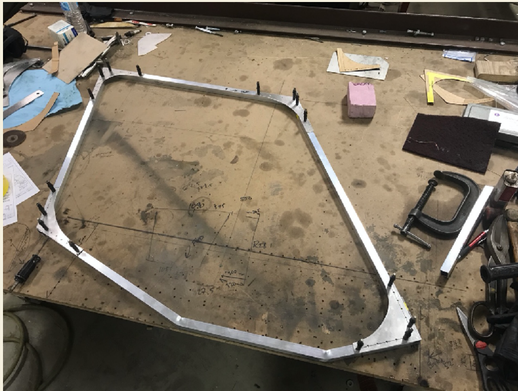
Presidential CH750 by Todd Scruton Door Frame Rebuild
